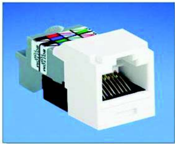
Figura 3. Jack RJ – 45 conector (TIA, 2009)
