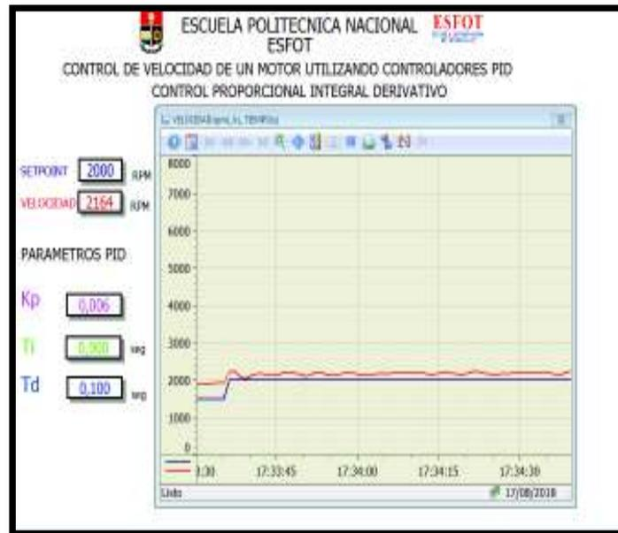
**Figura 3.59** Control (PID) con  $K_p = 0.006$ ,  $T_i = 0.90\text{seg}$  y  $T_d = 0.10\text{seg}$  a 2000 rpm
