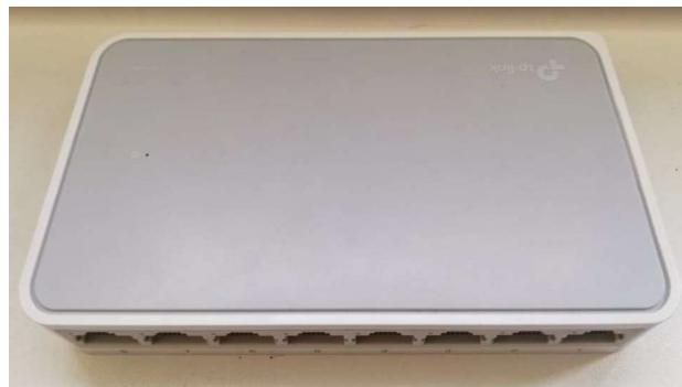
Figura 2.17. Switch TP-link TL-SF1008D
