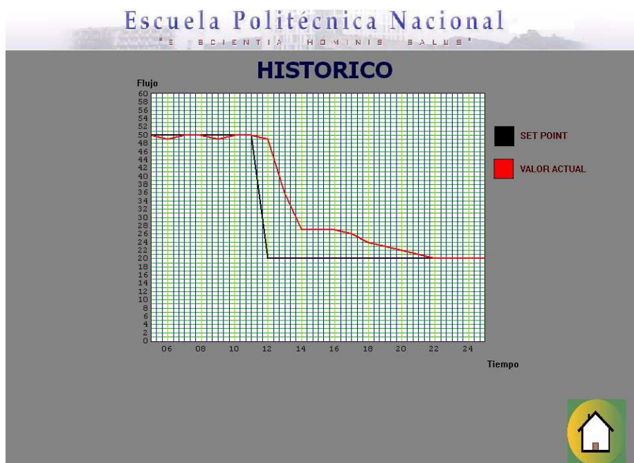
Figura 5.6 Valores de T_i=0.025 y T_d=0.0 , K_p=0.5 , T_s = 10 [s].
