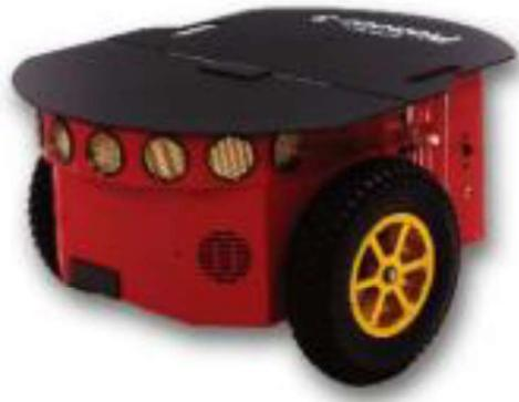
**Figura 1.1** Robot Pioneer 3-DX [3].
