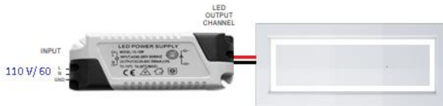
Figura 2.5. Conexión driver ON/OFF a Paneles Led
