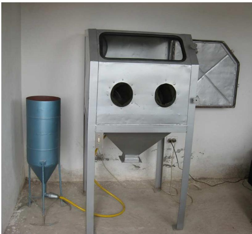
Figura 5.1 Cabina sand blasting.
