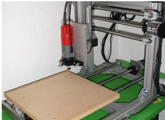
Figura 3.2 Modelo base CNC Router Aluminium
