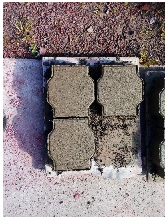
Figura 22 adoquín hexagonal 24X22X8
