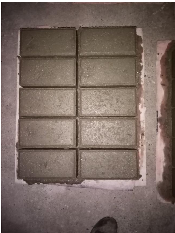
Figura 21 adoquín rectangular 20X10X6
