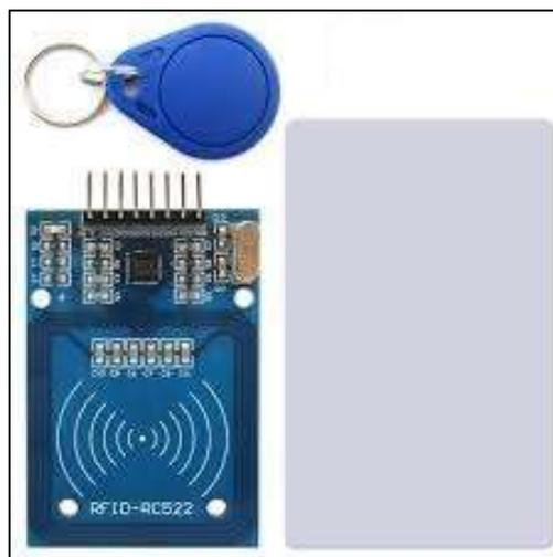
Figura 1.1: Módulo RFID-RC522 RF [1]
