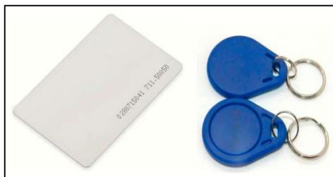
Figura 3.1: *Tag* RFID 13.56 MHz [1]
