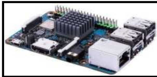
Figura 3.3: ASUS Tinker Board S [46]
