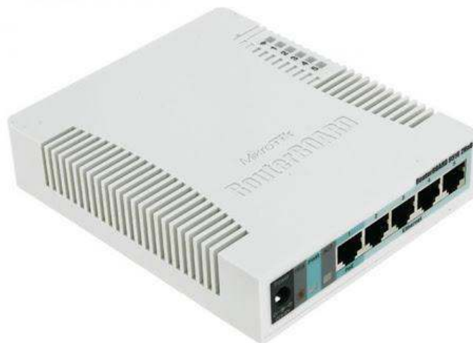
Figura 3.3 RouterBOARD RB951G-2HnD de MikroTik
