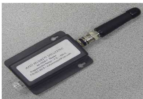
AA-R500SP Reader with AA-SANT Antenna
