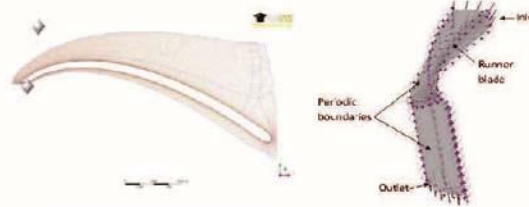
Fig. 10 TurboGrid ATM mesh
