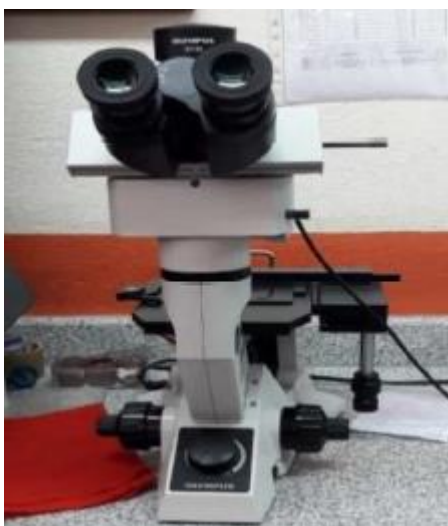
Figura 2.33. Microscopio Olympus GX441F.
