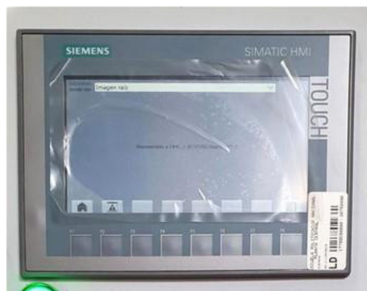
Figura 3.26 Vista frontal pantalla HMI KTP700 Basic.
