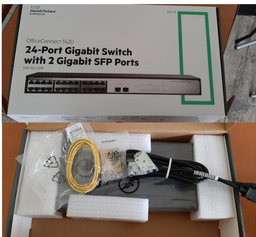
**Figura 3.22** Switch HP Enterprise HPE-1420-24G 1 adquirido
