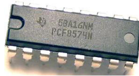
Figura 3.14 Circuito integrado expensor PCF8574 [23].
