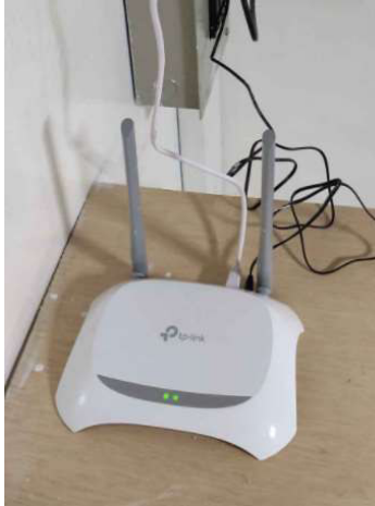
Figura 2.4 Router repetidor TP-LINK
