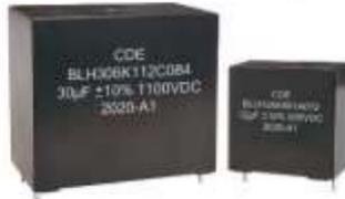
Type BLH DC Link capacitors use the most advanced construction and technology to meet the challenges of harsh environments. Tested for 1,500-hour at 85 °C / 85% relative humidity with rated voltage applied (50% greater than competitive THB test life). The series is qualified to automotive-grade electrical and mechanical testing per standard AEC-Q200.
