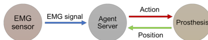
Figure 3.4 Communication diagram between devices
