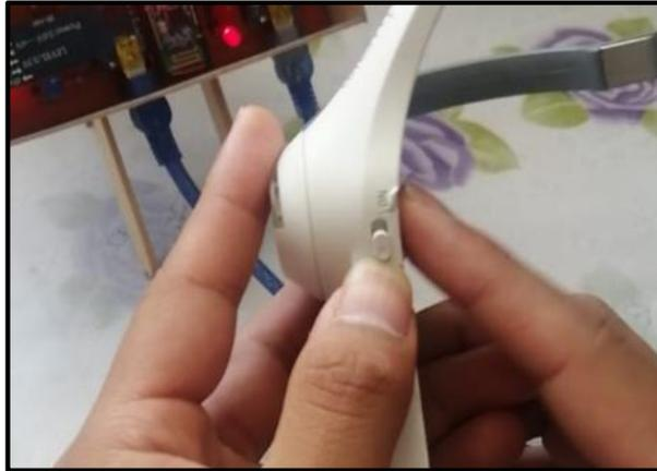
**Figura 3.26** Interruptor *On/off* de diadema *Mindwave Mobile*
