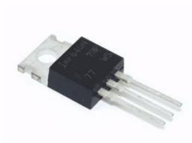
**Figura 2-75** Transistor de Campo IRF640.
