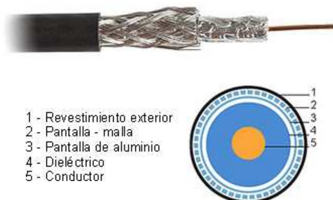
Figura 2.8 Estructura Cable Coaxial RG-59. [F8]
