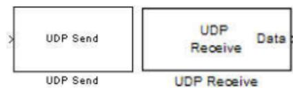
**Figura 1.8** Bloques de control UDP Send y Receive de Simulink [30].
