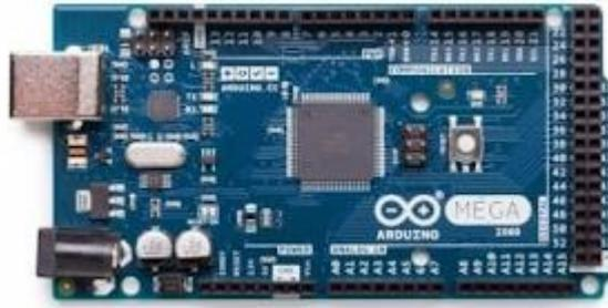
**Figura 2.8.** Arduino Mega 2560 [13].
