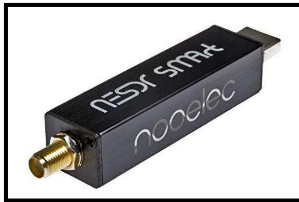
Figura 1.16. RTL-SDR NESDr Smart [69]
