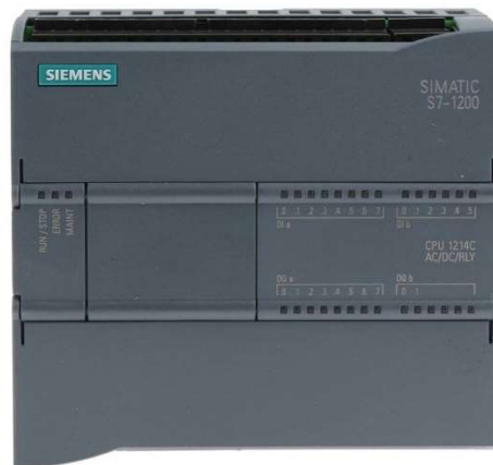
Figura 2.9 PLC Siemens S7-1200 CPU 1214C AC/DC/RELÉ
