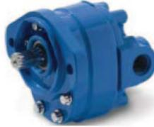
**Features:** 13-tooth gears minimize the flow ripple for reduced noise and vibration. Bearing lubrication system uses inlet oil instead of high pressure oil, improving volumetric efficiency. Innovative wear plate permits simple rotation change.
