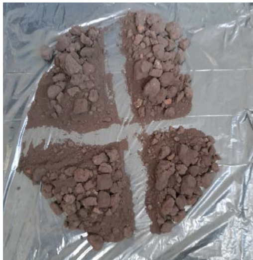
Figure TS1.1. Sample size reduction through quartering.
