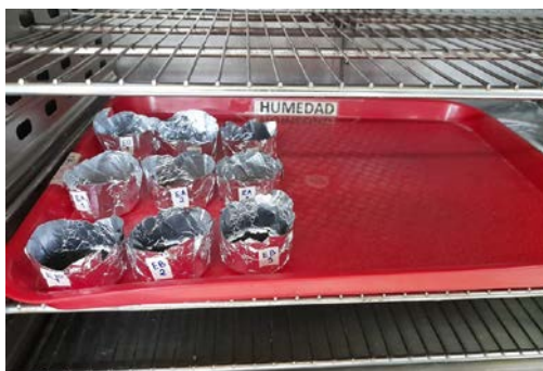
Figure TS2.1. Moisture content analysis evidence.
