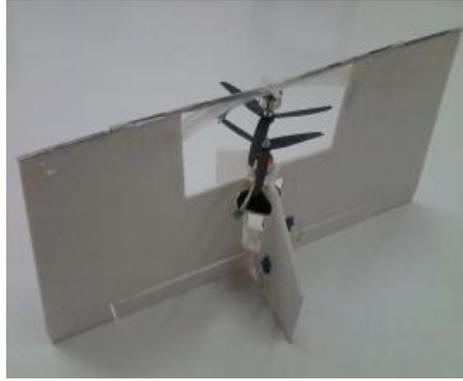
*Fig. 4 Tail Sitter - Coaxial Dual Rotor.*
