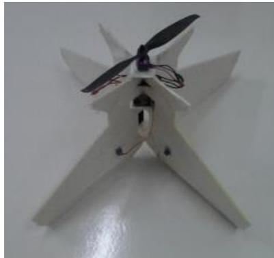
*Fig. 3 Tail-sitter - Single rotor.*
