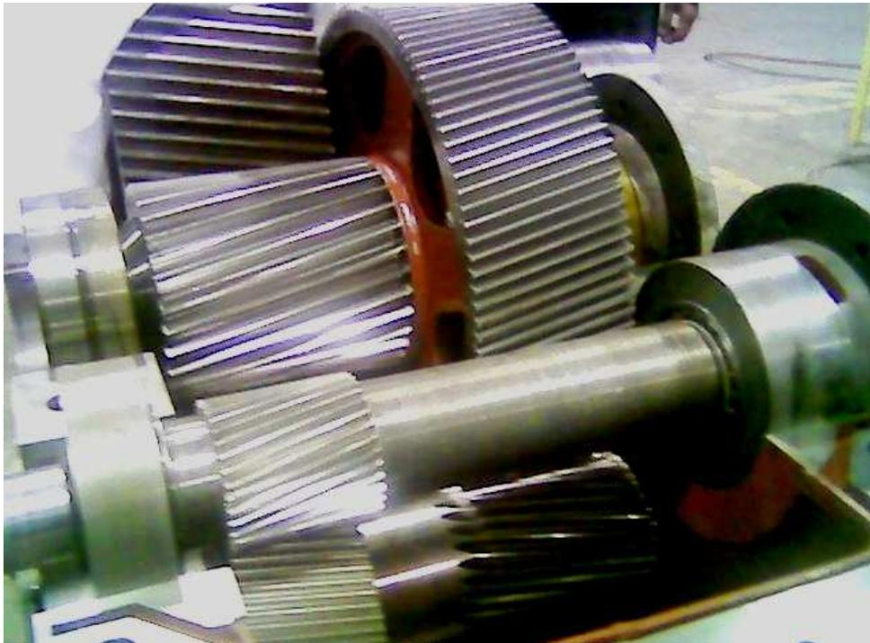
FIGURA 2.6 REDUCTOR PRINCIPAL DEL HORNO DE LAFARGE
