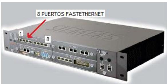
Fig. 16 Vista frontal del multiplexor HiT7030
