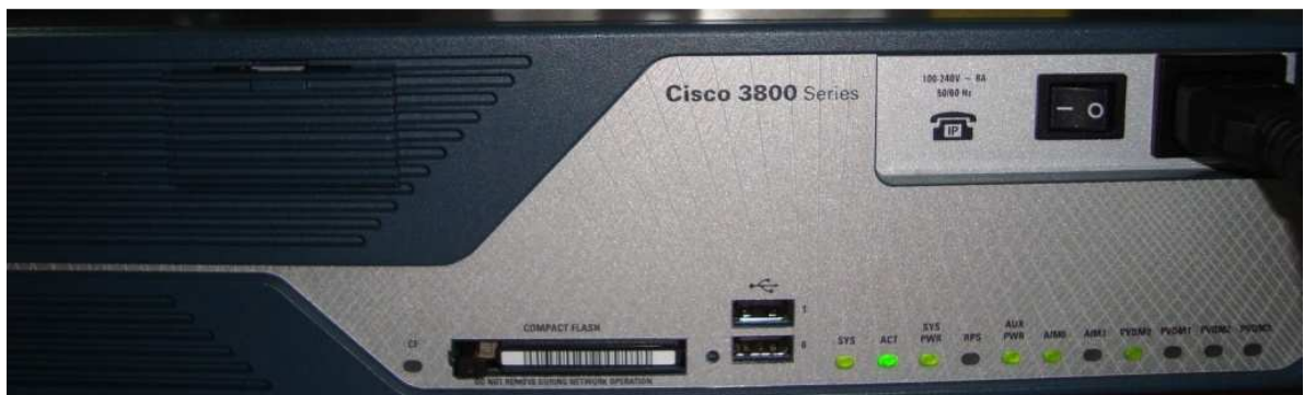
Figura 4.47 Router Cisco 3825 vista frontal
