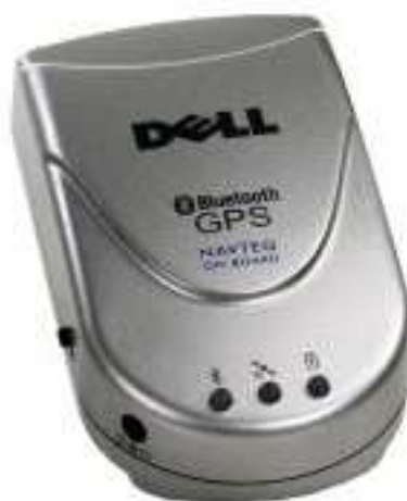
Figura 2-10. GPS-Bluetooth DELL NAVTEQ ON BOARD Modelo BT-309
