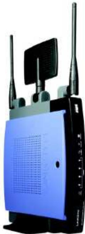
The Wireless-N Broadband Router is really three devices in one box. First, there's the Wireless Access Point, which lets you connect to the network without wires. There's also a built-in 4-port full-duplex 10/100 Switch to connect your wired-Ethernet devices together. Finally, the Router function ties it all together and lets your whole network share a high-speed cable or DSL Internet connection.
