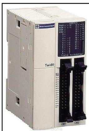
**Figura 2.15.** PLC Twido TWDLMDA40DTK.
