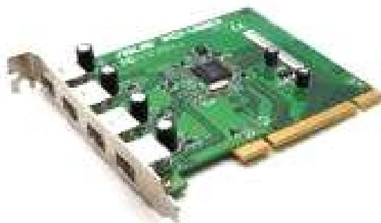
*Figura 2.7 Tarjeta PCI-USB 2.0<sup>1</sup>*
