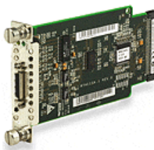
Figura 4-9: Tarjeta 3COM 1 puerto serial
