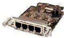
Figura 4-43: Módulo Cisco 4 puertos FXS/DID
