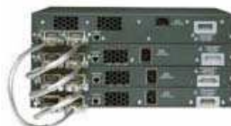
Figura 4-28: Cable Cisco StackWise 50 cm
