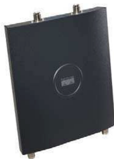
Figura 4-38: Access Point Cisco Aironet 1242AG
