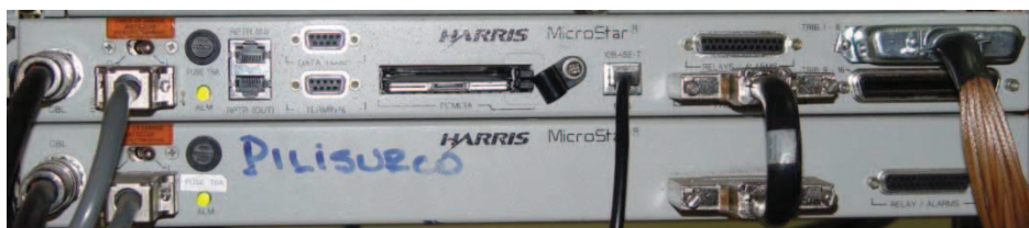
Figura 2.6. Radio Harris MicroStar [2.9]
