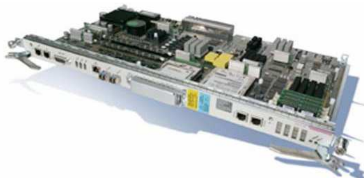
Figura 2.10: Tarjeta Route Processor [19]
