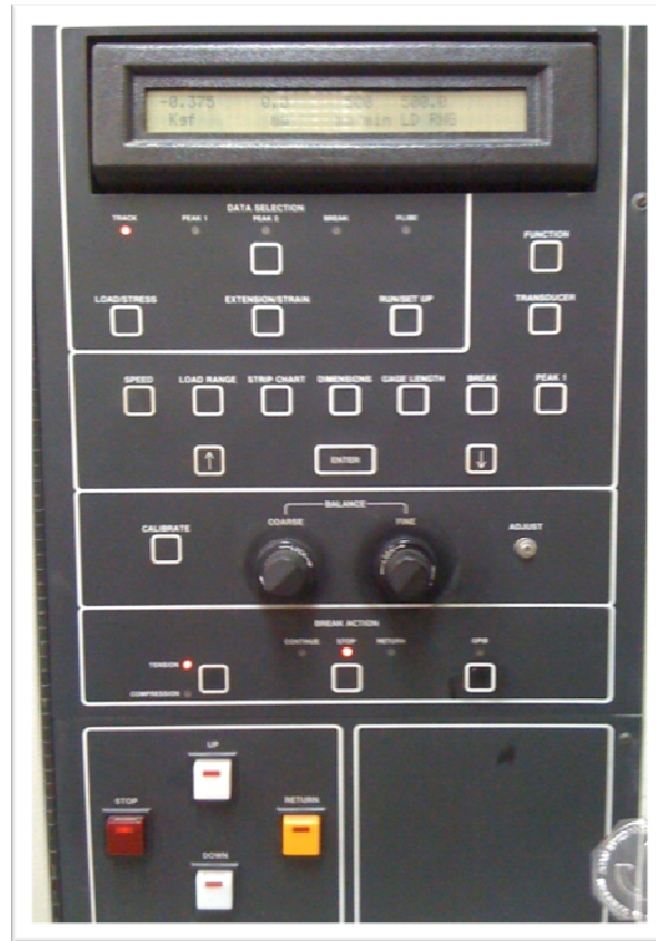
FIGURA 1-2. Panel Frontal INSTRON 1011 AMTS
