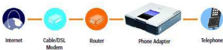
Figure 3-1: Connect the Phone Adapter to Your Network and Telephone
