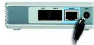
Figure 3-4: Connect the Power
