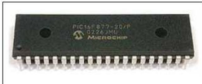
Figura 2.4 Microcontrolador PIC 16F877A<sup>1</sup>
