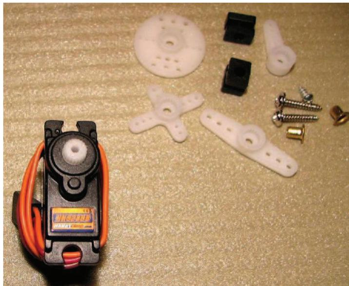
Figura C- 3 Servomotor HK928BB
