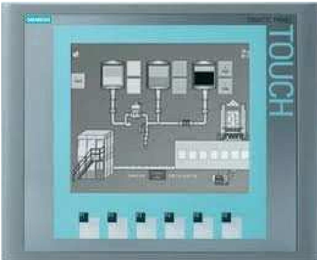
**Figura 2.26: Panel View KTP600 BasicMono de Siemens**
