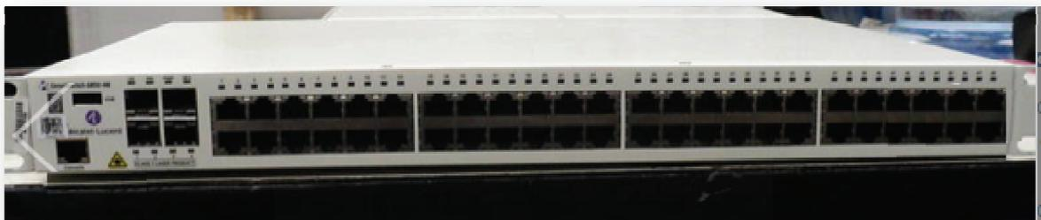
Figura 3.27 Switch Omniswitch 6850-24L
