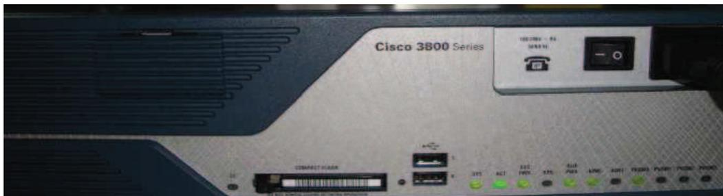
Figura 3.17 Router Cisco 3825 vista frontal
