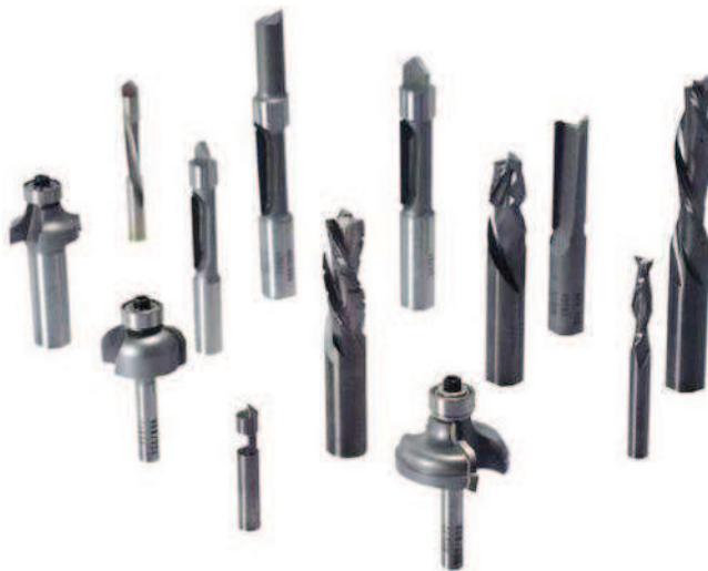
Figura 3.70 Fresas o router bits.
