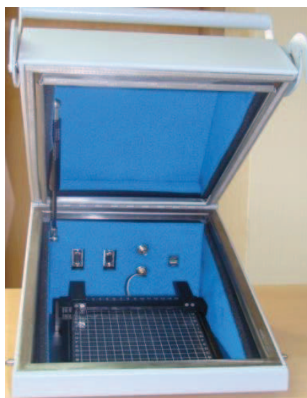
Figura 3.9 RF shielded box, Jaula de Faraday
