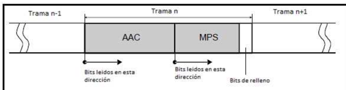
Figura 1.11: Trama AAC + MPS
